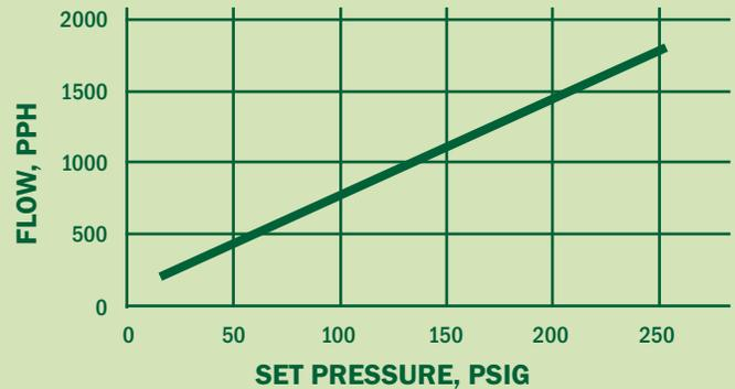
"D" Orifice - 1/2" through 1" NPT Inlet
